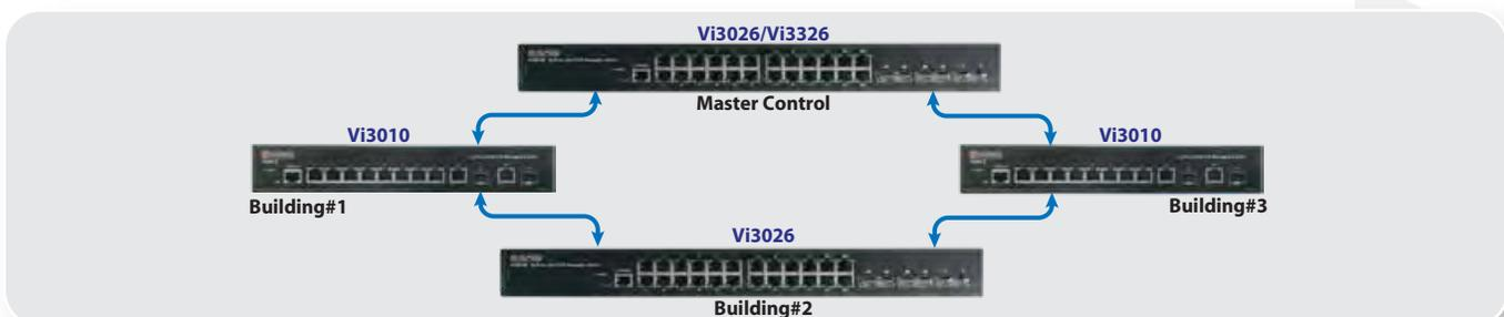
Selected Vigitron managed switches offer Virtual Auto Stacking, allowing use of a single IP address to control and monitor several switches on the same network without location restriction. It also eliminates the need for special stacking cables.
