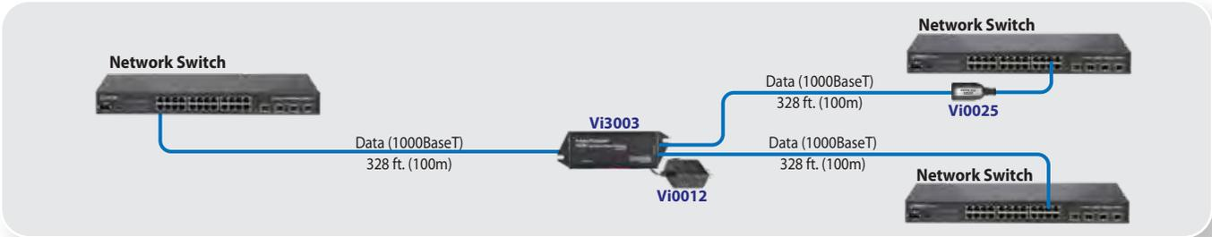
The Vi0025 blocks PoE when “Always On” PoE ports are connected to non-PoE ports.
