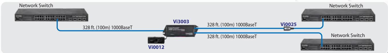
The Vi3003 enables 1G connection between network switches eliminating the need for using fiber optics.
