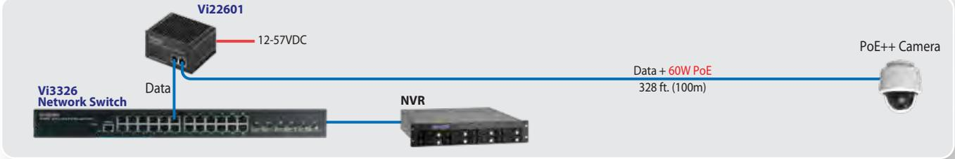
The Vi22601 is a compact and high power Midspan with 12VDC or 48-57VDC input that can provide PoE++ up to 60W for a wide variety of high power applications.
